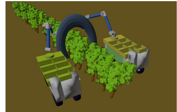
Confined biocontrol spraying/lighting
